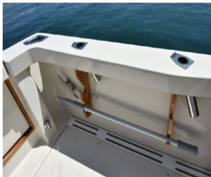
pozzetto con ampie griglie per svuotamento rapido. self draining cockpit with large scuppers and gutters for quick drainage of water and debris.
